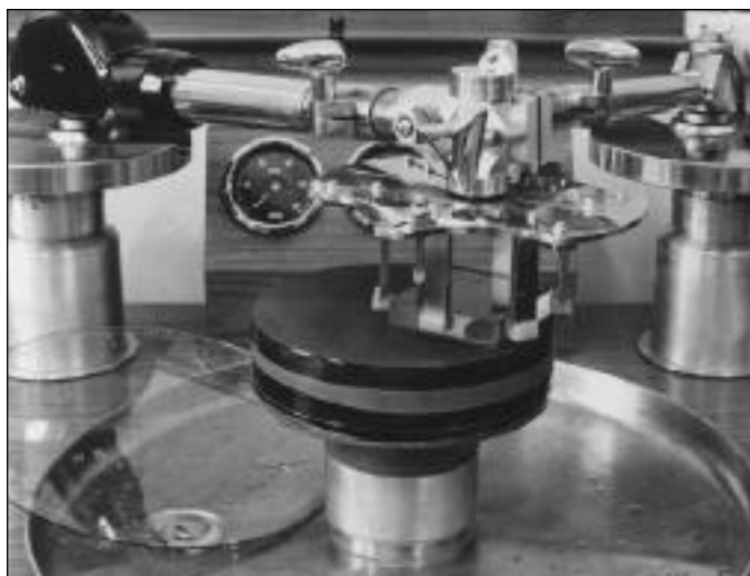
A photograph in the Bill James archive – polishing a square component on a Teflon polisher with the special holder.
